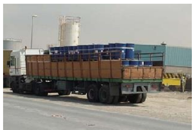
Unsafe Securing Arrangement
